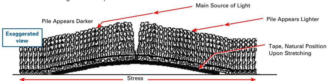
To verify that an apparent shade difference is caused by seam peaking, the seams should be viewed with a powerful overhead light while all side lighting is eliminated. When conducting such a test on a cut pile carpet, ensure that the pile is brushed in a consistent direction on both sides of the seam.
