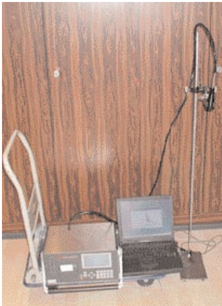
Test set-up for an indoor air measurement
