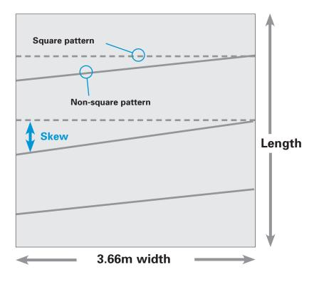
Should **Hooked Edges or Hooked Edges in combination with either Bow or Skew occur** resulting in wavy or crooked pattern lines, tolerances as noted for Bow and Skew are applicable.
